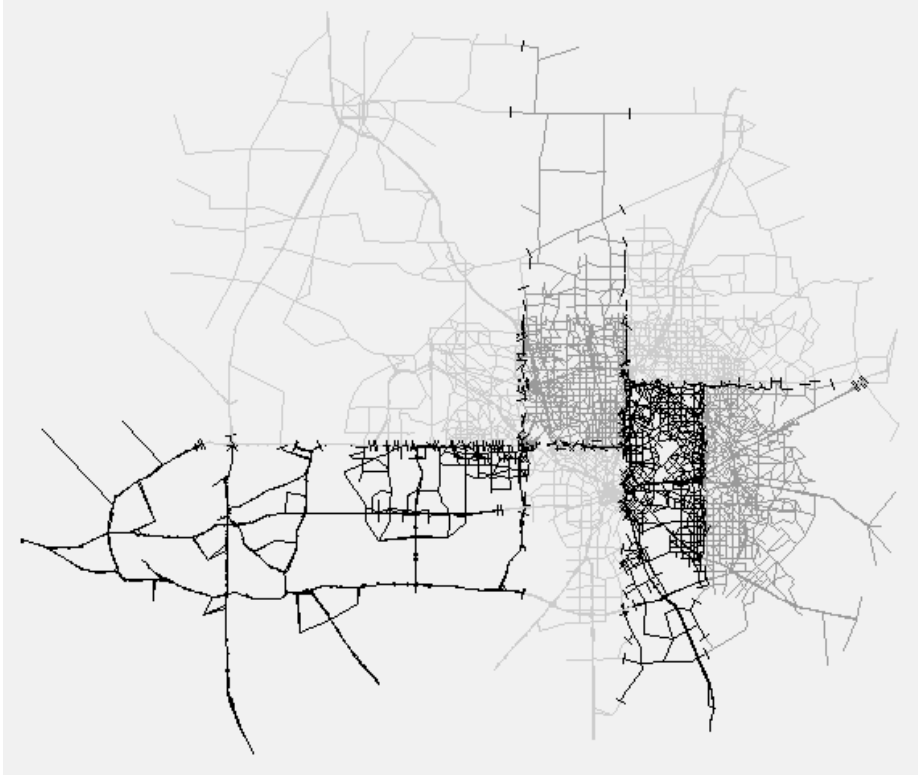
Fig.5. Domain decomposition example for 7 workstations. On the right is Dallas; for Fort Worth on the left only the major arterials are included. The corresponding microsimulation runs faster than real time.
